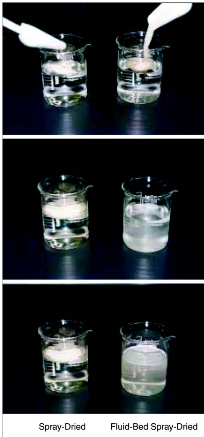
Figure 4. Dispersibility of the protein powders produced by spray drying (left) compared to the protein powders prepared by fluid bed spray drying process (right).
